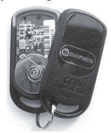
Locate the recess near the keyring and using a small coin or flat blade; gently prise apart the two halves of the Radio Key casing.
