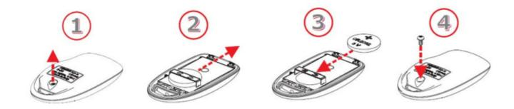
Please note: Battery type – CR2032. Different battery types can seriously damage the remote control. Discard used batteries properly in special dedicated containers.
